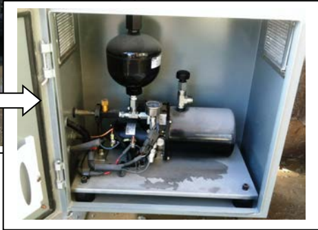
Custom built hydraulic power unit, 24VDC
