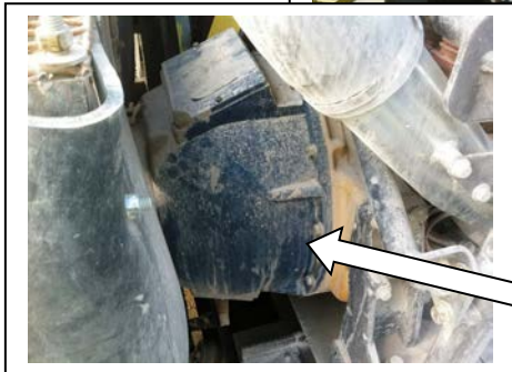
Custom built hydraulic power unit, 24VDC
